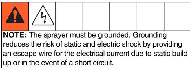
The sprayer cord includes a grounding wire with an appropriate grounding contact.
