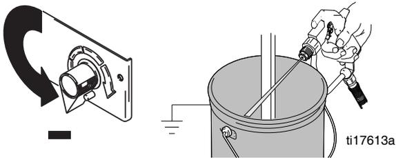
4. Put drain tube in pail. Turn prime valve down to DRAIN position.
