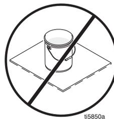
**Grounding a metal pail:** Connect a ground wire to the pail by clamping one end to pail and other end to a true earth ground such as a water pipe.
