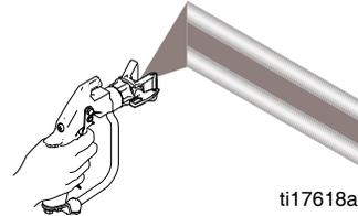
2. Hold gun perpendicular, 10-12 in. (25-30 cm) from surface. Spray back and forth. Overlap by 50%. Start moving the gun before triggering and release trigger before gun stops moving.
