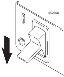
2. Lock gun trigger safety. Remove guard and tip.
