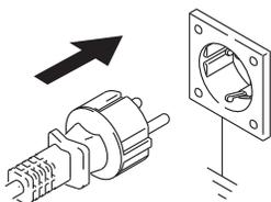
Do not modify plug! If it will not fit in outlet, have grounded outlet installed by a qualified electrician. Do not use an adapter.
