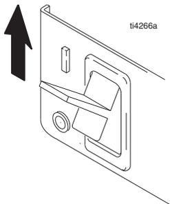
3. Increase pressure 1/2 to start motor and allow fluid to circulate through drain tube for 15 seconds; turn pressure down.
