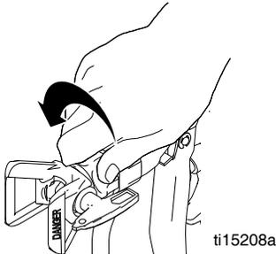
3. Turn pressure to lowest setting. Trigger gun to relieve pressure.
