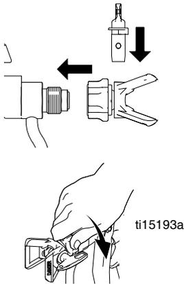
3. Screw assembly onto gun. Tighten.
