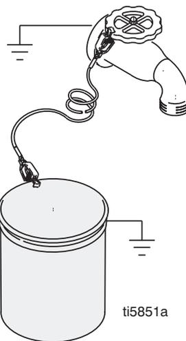
**To maintain grounding continuity when flushing or relieving pressure:** Hold metal part of spray gun firmly to side of a grounded metal pail. Then trigger gun.
