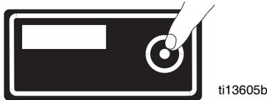
2. Turn pressure to lowest setting. Trigger gun to relieve pressure. Turn prime valve to drain position.
