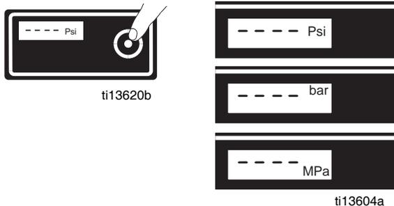
2. Short press DTS button to move to Job Gallons (or liters x 10). **Note: JOB** displays briefly, then the number of gallons sprayed above 1000 psi (70 bar, 7 MPa) displays.
