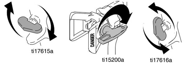
2. Put safety ON. Return tip to original position. Take safety OFF and continue spraying.
