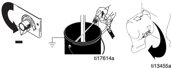
3. Turn power ON. Pressure display appears. Dashes will appear if pressure is less than 200 psi (14 bar, 1,4 MPa).
